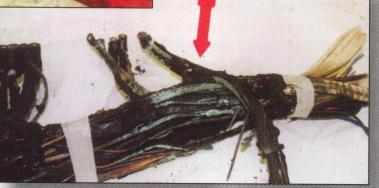
When one wire overheats, others in the same bundle can ignite. Not having proper fusing during a battery charger malfunction caused most of this boat's wiring to be damaged—a daunting repair (claim #0100202).
