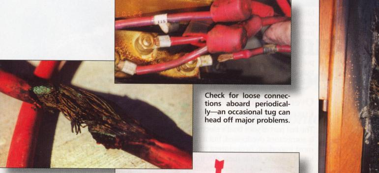
Starter cables carry a lot of electricity. This cable wasn't supported with cable clamps in the engine room and abraded against a spinning shaft. The subsequent fire began destroying the engine control cables and after the member shut down the engine, it restarted. The kill switch wiring was damaged and the engine had to be stopped by choking the air supply (Claim # 9605729).
